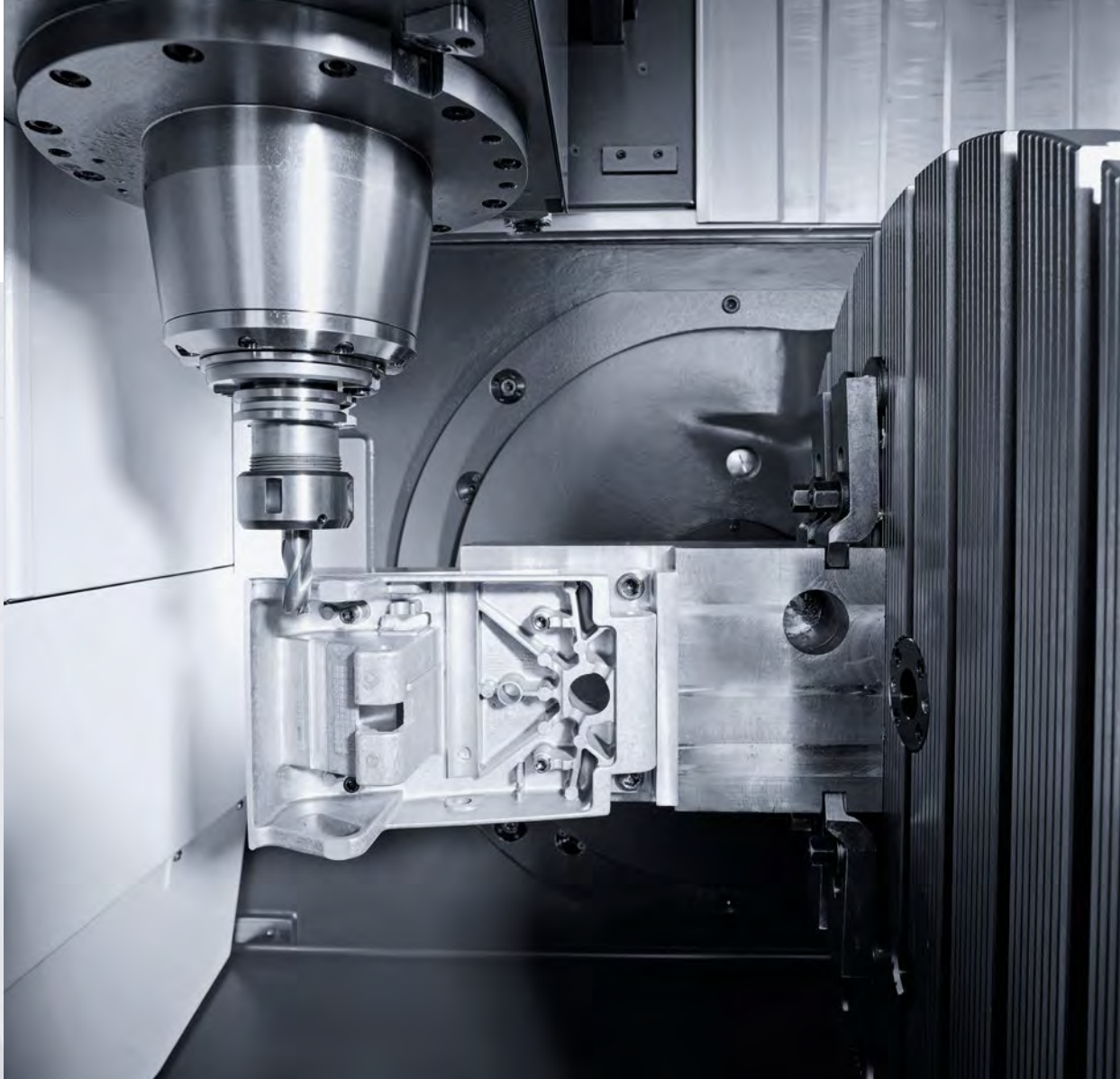
Hydraulic table clamping and maximum table load up to 350 kg (CMX 70 U)
